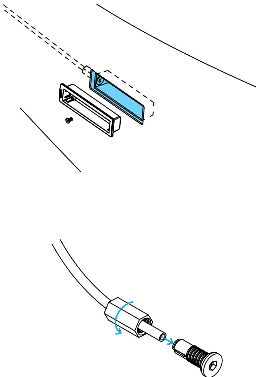
**B. Installing the skeg control 4 box and connector tube in the open surface recess or retrofit without any recess by using the KS-adapter box for skeg control 4.**
